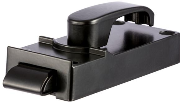
Designed for compartment and access doors where low cost slam action latching with L-handle actuation is desired. It features a robust zinc die cast plunger bolt for durability.
